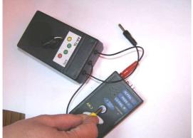
Plug red banana plug of the AR-CAL.CHECK Calibration Checker into left, red socket of the AR-7 tester. B1. Connect Calibration Checker with AR-8 Wrist and Footwear Tester
