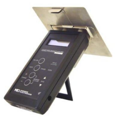
\* Two rubber feet are included with the plate. Apply to the two front corners of the battery compartment on the rear of the unit to stabilize placement of the meter when being used in the horizontal position.
