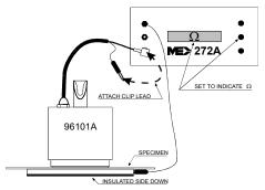
Figure 3: Setup for <u>Guarded</u> Measurement of Volume Resistivity
