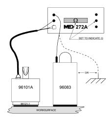
Figure 2 Setup for Surface-to-Ground and Surfaceto-Surface Resistance Measurements
